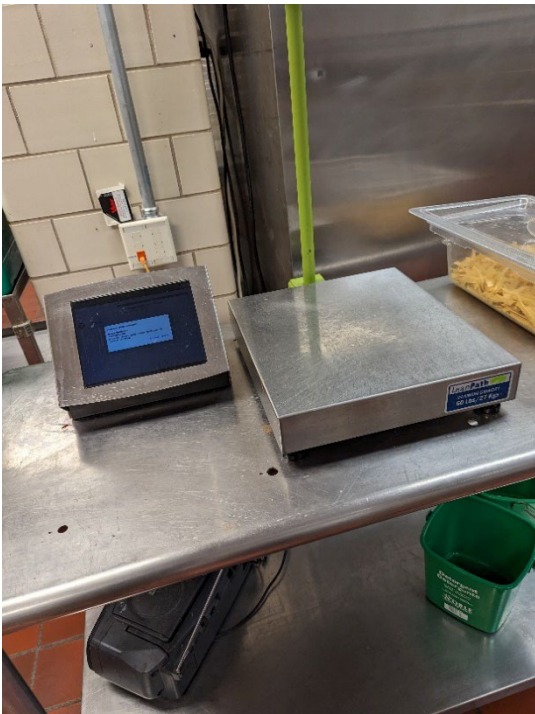
Figure 25. Leanpath system of scale and camera on a counter in a campus dining hall kitchen.
